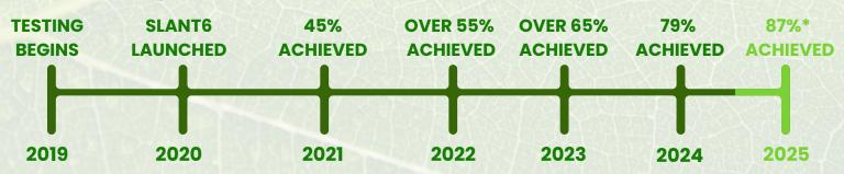
Independent long term testing at Eden Research Laboratory in the USA to the ASTM D 5511 test standard. This test simulates landfill conditions.
